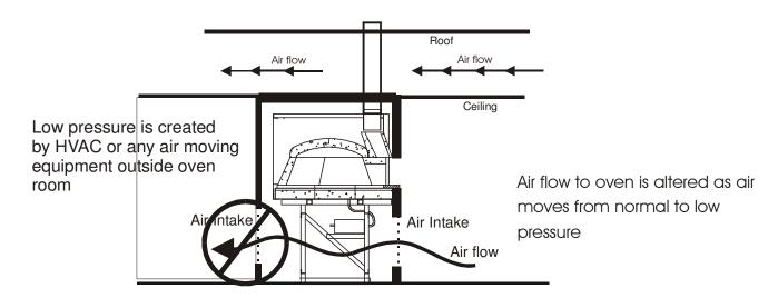
In this case the air intake located on the rear of the oven should be closed.
