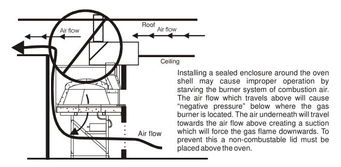
3) Altered air flow from air intake in a separate room with low pressure.
