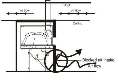
In this case a 24"x24" opening will be needed for proper air combustion.
