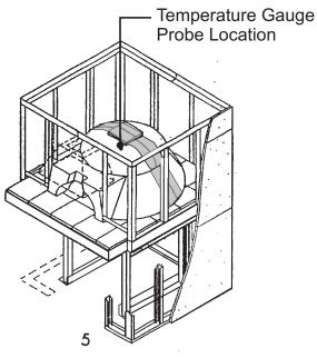
6. Insert metal conduit for temperature probe in the pre-drilled hole located on top of the oven dome. Cover top of conduit with a piece of masking tape. This will prevent insulation and other particles from entering into the hole. Fill the void between the oven and outer enclosure with the insulation mixture as specified. Insulation should cover 4 inches above the oven dome. Make sure to follow oven curing directions in the installation instruction booklet.
