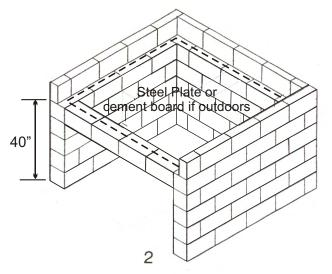
3. Place plywood form to make front shelf. Follow with positioning ½ inch plywood strips (supplied) around perimeter of 6th course to create expansion joint. Make sure to oil plywood to prevent moisture build up and to prevent sticking of concrete. Lay horizontal rebar. Pour 4 inch thick concrete slab. Remove plywood strips 2 hours after slab has been poured. Allow concrete to set for 24 hours before installing hearth tiles.
