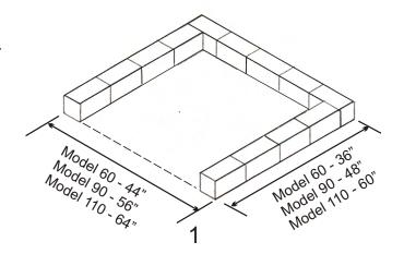
2. Set the first five course of block. Place vertical and horizontal rebar as specified in installation instructions. Lay 1/16 inch steel plates in position (cement board can be used in outdoor applications in place of steel plates). Bend rebar over insulation until parallel. Install 6th course of block. Courses of block can be added or subtracted to accommodate 40" different hearth levels.
