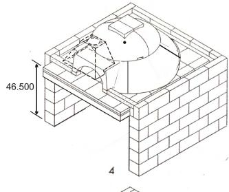
5. Seal all joints on oven with supplied bag of high heat refractory cement. Follow by placing metal flashing over joints as specified in installation instructions. Set the last courses of four inch block and the courses around the front entrance piece. Fill the cells of the block with concrete. Make sure the top is filled and finished smoothly. Place conduit for temperature gauge probe in the pre-drilled hole.
